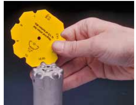
A useful tip: use a Secoroc grinding template, and you'll see when it's time for a regrind.
